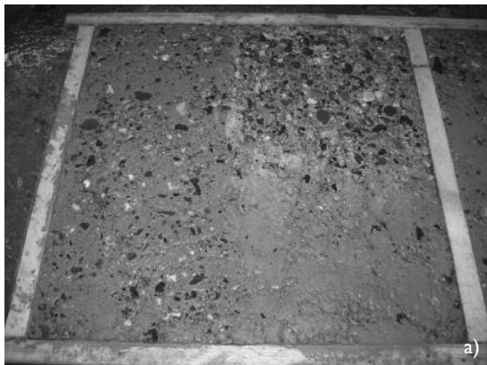
Fig. 4 To reproduce the eroded facies encountered on the ancient concrete to be restored, two deactivation products were tested, inducing 2 depths of deactivation (a) and (b).
