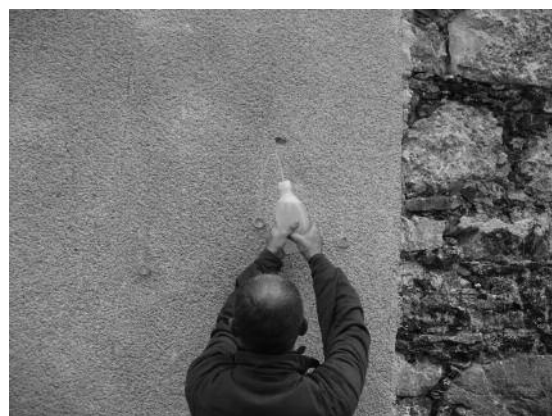
Fig. 7 Water absorption tests on rendering layers.
