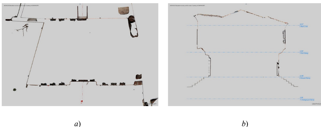
Figure 3. Sections through the point cloud in ArchiCAD: a) horizontal at height 1,20 m; b) vertical 1-1, depth 10 cm.
