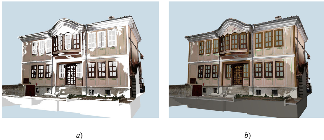
Figure 4. 3D volumes superimposed over the point cloud: a) white colour; b) contrasting solid colour.
