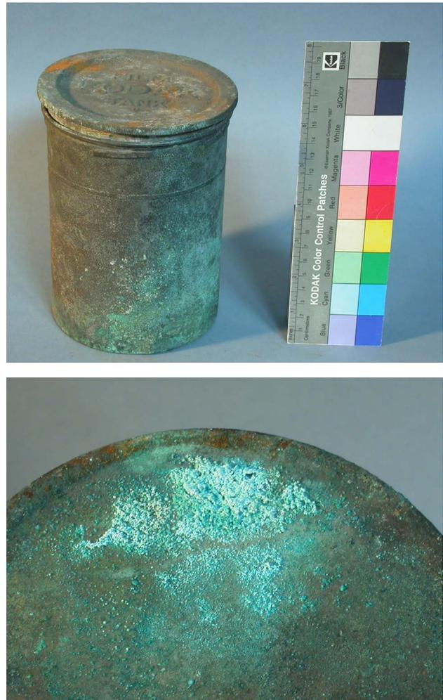
**Figure 2.** a) Kodak developing tank in copper alloy from MUHNAC; b) detail of the surface corrosion (photo: Manuel Lemos; courtesy MUHNAC, University of Lisbon).
